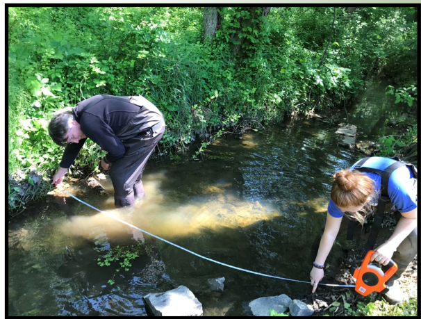
Jim Walter, Penn State Master Watershed Steward, and Ashlin Brooks, BCCD Summer Intern, measure channel width at a sampling site on a Poquessing Creek tributary in May 2019.
