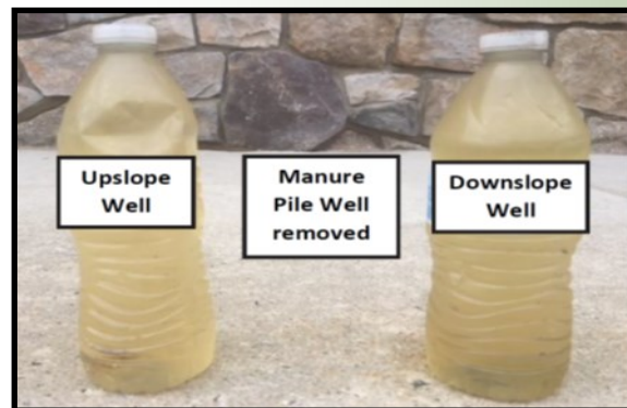
AFTER: Farm #1 after a roofed stack pad was installed at the same location. Groundwater samples are from 2 months after the roofed stack pad was installed.
