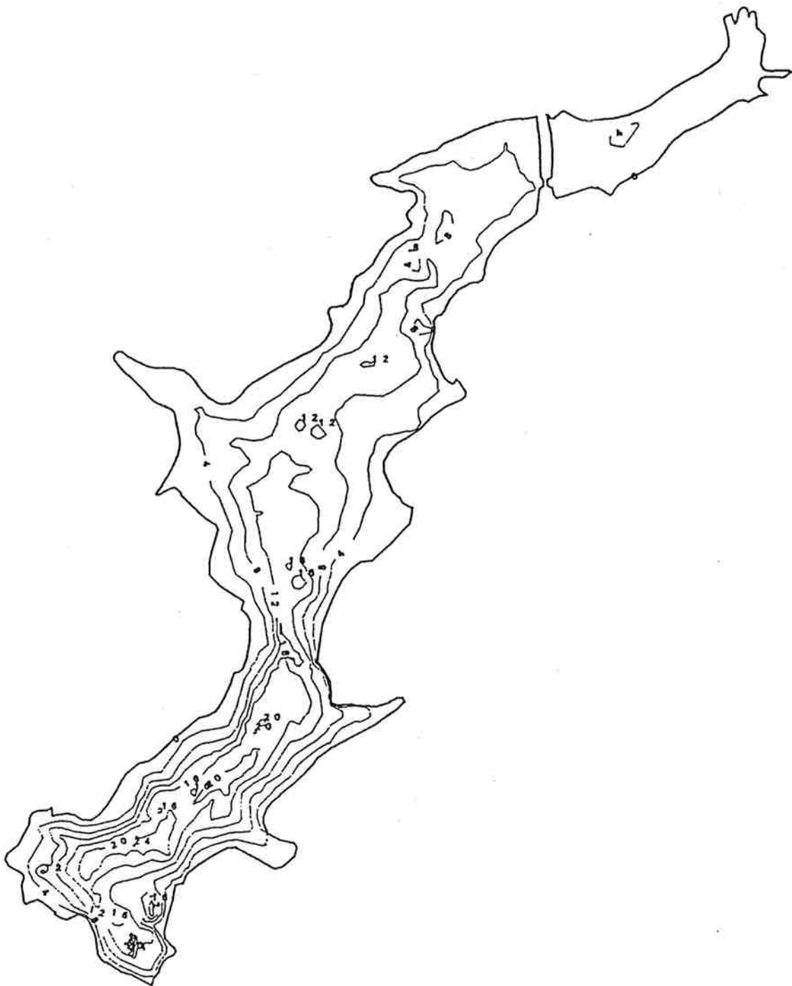
Figure 2.1 Bathymetric Map of Lake Luxembourg Scale: 1" = 1000' Contour Interval = 4'
