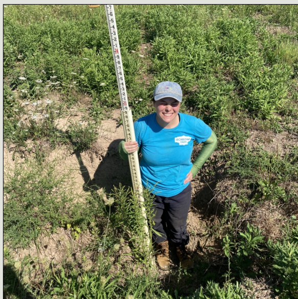
Carly, one of our ACTs, is measuring the depth of erosion in a cropland gully from seeps, a huge resource concern .
